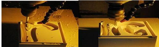
Figure 3: Plaster Moulds created with CNC
