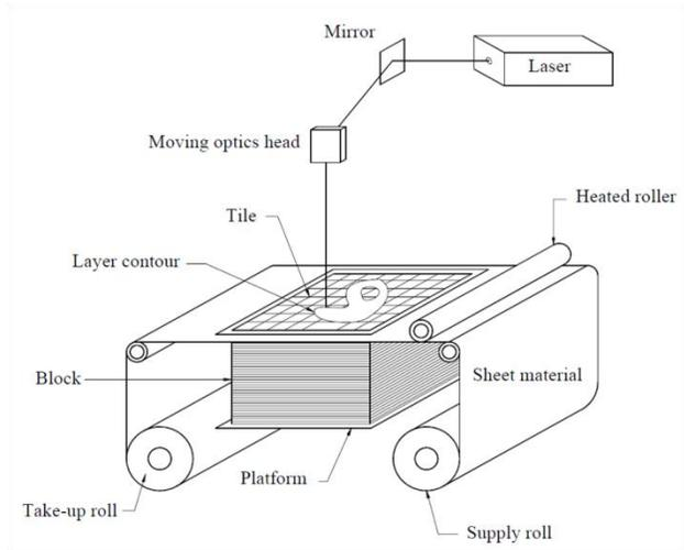
Figure 2: Illustration of the working principles of LOM
