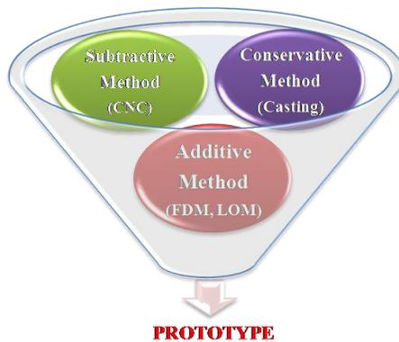
Figure 1: The three different ways of creating prototypes
